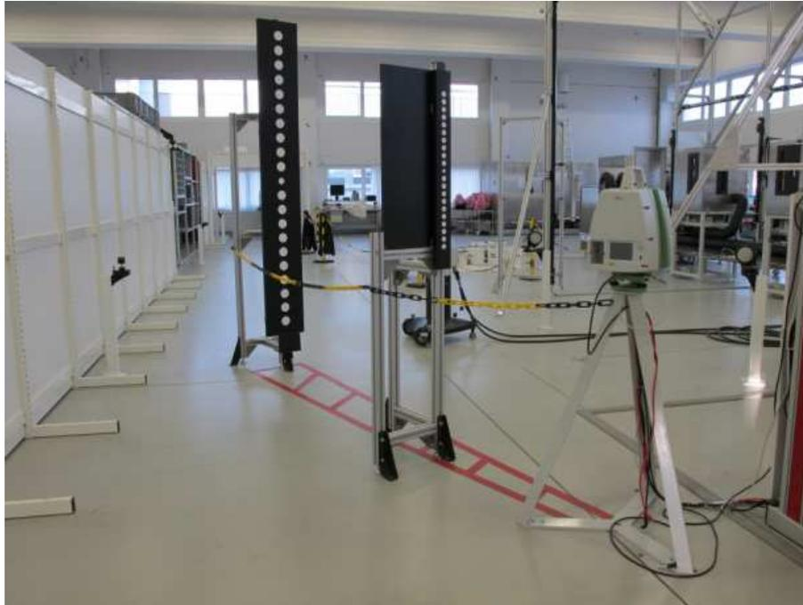
**Figure 8:** A view of the camera calibration stand. Two sets of targets are placed in front of the scanner and are both imaged and scanned.
