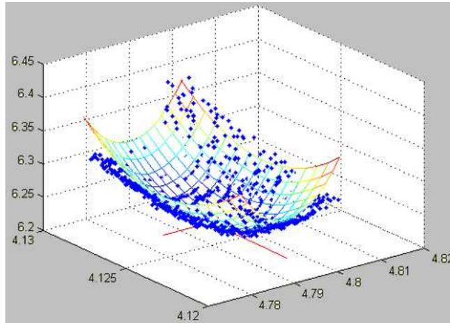
**Figure 6:** Example fit of a laser scanner scan of a tracker ball. Plot is generated by MATLAB and algorithm is by the author. Calibration process is run by a MATLAB script.
