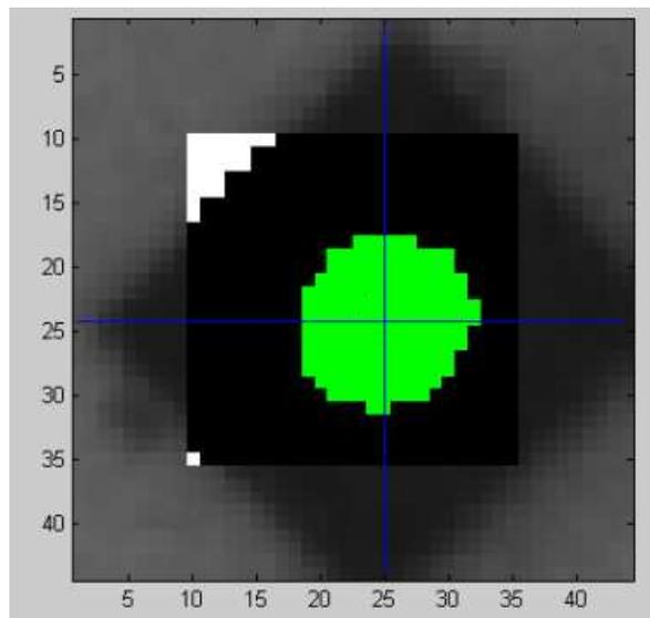
**Figure 13:** A match between an image center and a LIDAR determined center. The scanner locates the target, and then the camera image is taken. The image is turned into a black and white image, and put through a center extraction algorithm to determine the center. Pixels which belong to the white disk at the target center are colored green by the algorithm, and the estimated image center is marked by the cross hairs.
