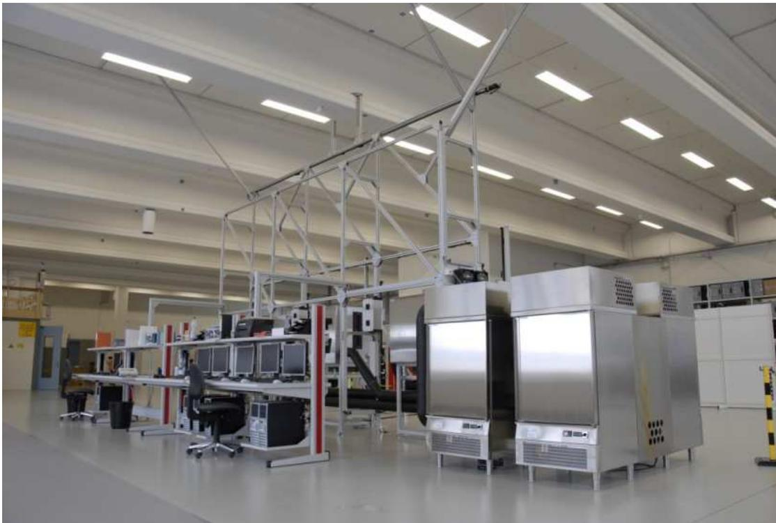
**Figure 4:** Operator view of the calibration chambers in Widnau. Thermal control units are connected via insulated air ducts to each scanner calibration chamber, allowing each chamber to be set at independent temperatures.
