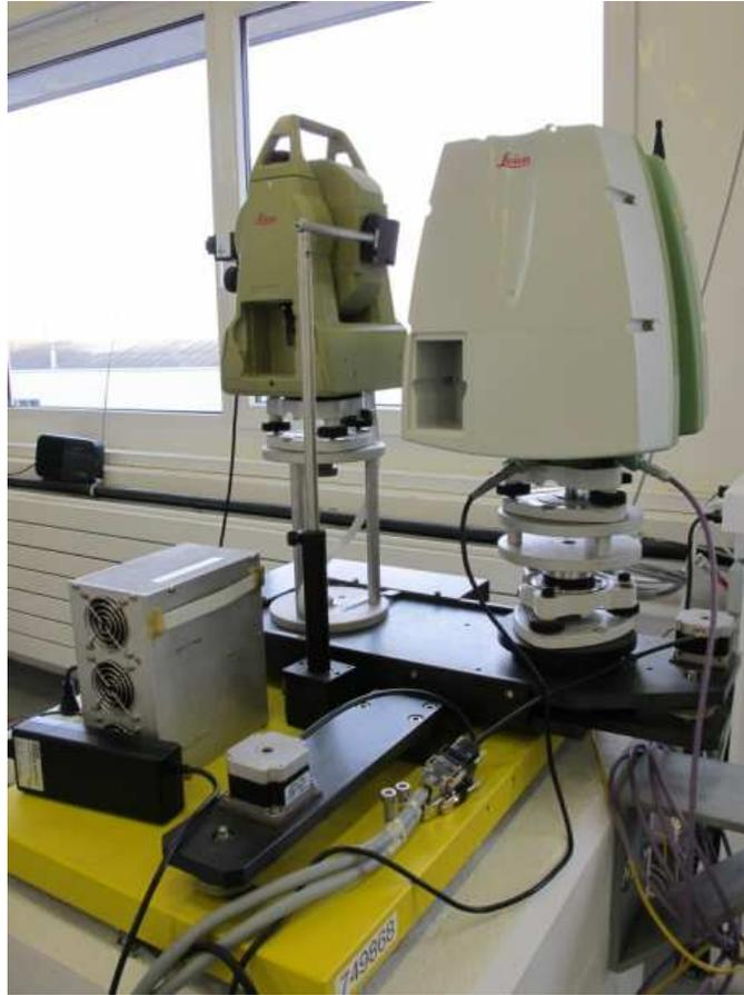
**Figure 7:** Tilt calibration station for the Leica ScanStation C10.
