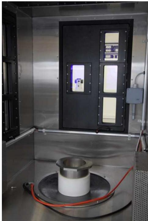
**Figure 2:** Inside view of Leica Geosystems Calibration chamber. From the front window the laser tracker reference system can be seen. The laser scanner mounts into the hard mount pedestal and the door of the chamber is sealed.
