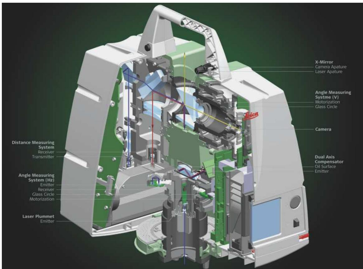
**Figure 1:** A cut away view of the Leica ScanStation C10, showing major components.
