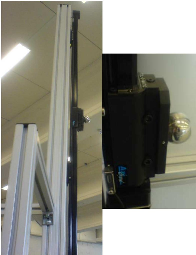
**Figure 5:** Motorized stage (left) with Leica tracker ball attached to magnetic mount (right, close up). The motorized stage allows the tracker ball to be moved and the target used many times in one calibration. With each scanner measurement, the position of the tracker ball is measured by the laser tracker to a high accuracy; the tracker measures the tracker ball's internal corner reflector. The scanner measures the outside surface.
