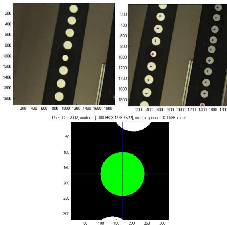
**Figure 9:** Images from a Leica C10 scanner as viewed in MATLAB. MATLAB has drawn on the image guess locations of the target centers using an approximate camera model. These
