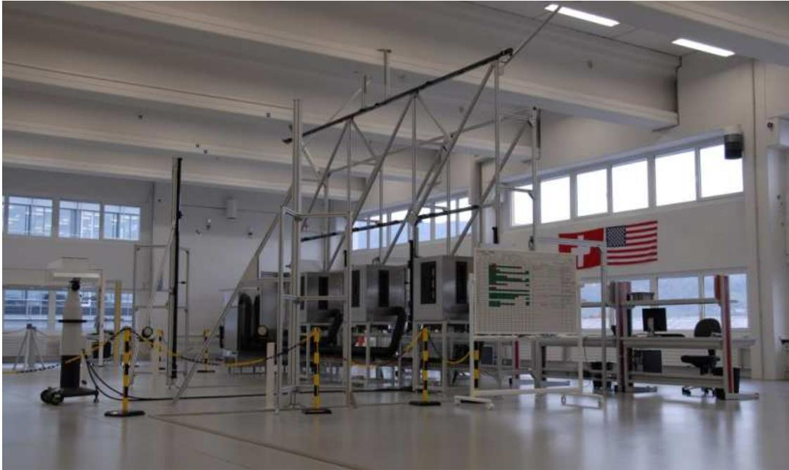
**Figure 3:** View of the calibration floor in Widnau, Switzerland. Three calibration chambers are visible in the photograph, as is the reference laser tracker. Three calibration chambers are also installed in San Ramon, California, USA.
